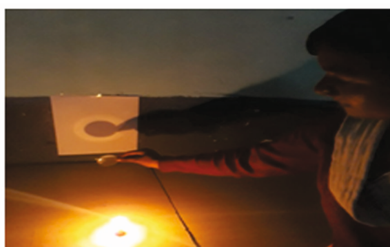
Figure 11.17 (b) : Images of objects placed at different distances using a convex lens.
