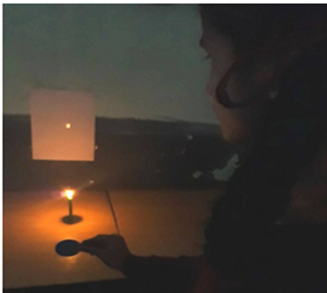
Figure 11.11: Image of an object on screen formed by a concave mirror
